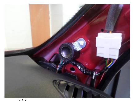
Note : Clip the small tab of the holder on the upper part, and the big tab on the lower part
