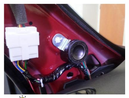
*Note* : Clip the small tab of the holder on the upper part, and the big tab on the lower part
