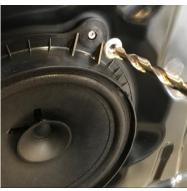
b. Remove the rivet's body from the inside
