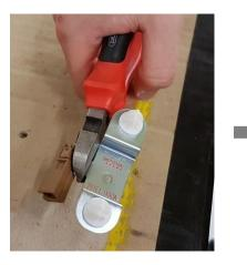
b. Screw back the tweeter putting a washer between the screw and the holder
