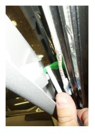
*Note* : The green clip must be rotated by one quarter turn in order to be removed
