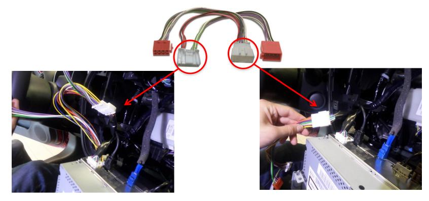
7 Wiring of the tweeters from the stereo a.Left tweeter
