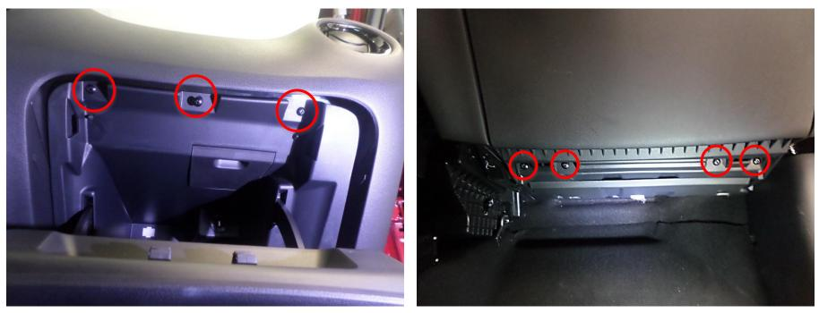
c. Right tweeter - Black and grey - remove the glove box then put the wiring underneath it
