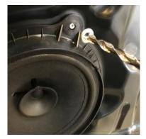
b. Remove the rivet's body from the inside
