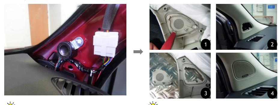
Note: Clip the small tab of the holder on the upper part, and the big tab on the lower part
