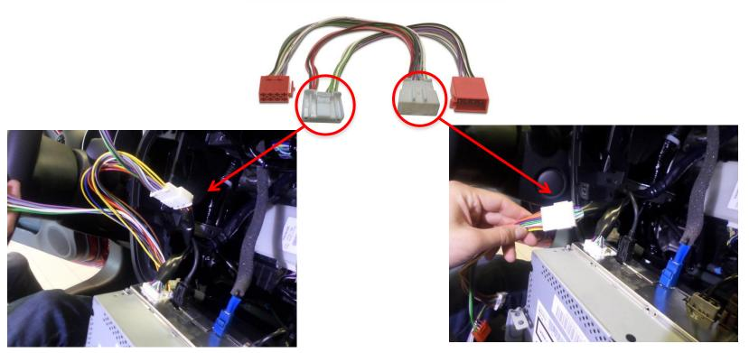
Wiring of the tweeters from the stereo
