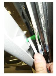
Note: The green clip must be rotated by one quarter turn in order to be removed
