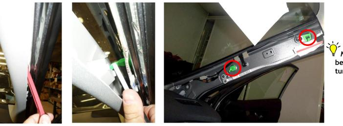
*Note* : The green clip must be rotated by one quarter turn in order to be removed
