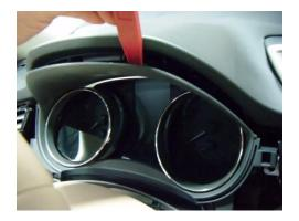
7 Remove the odometre
